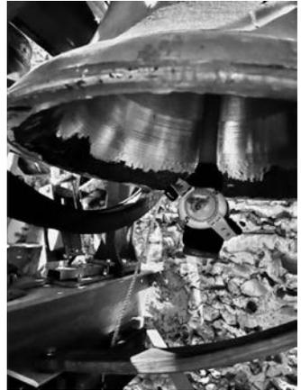
A leather muffle on a bell clapper dulls the sound of a strike to a poignant hum.
